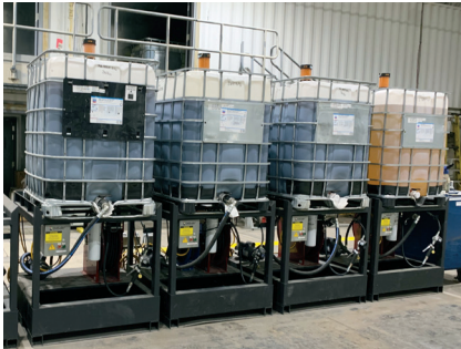
Storing bulk products in totes equipped with desiccant breathers is a Best-in-Class practice that helps reduce lubricant contamination. Pictured: Rolling stock shop before (below) and after (above) implementation of Chevron Site Assessment recommendations.
